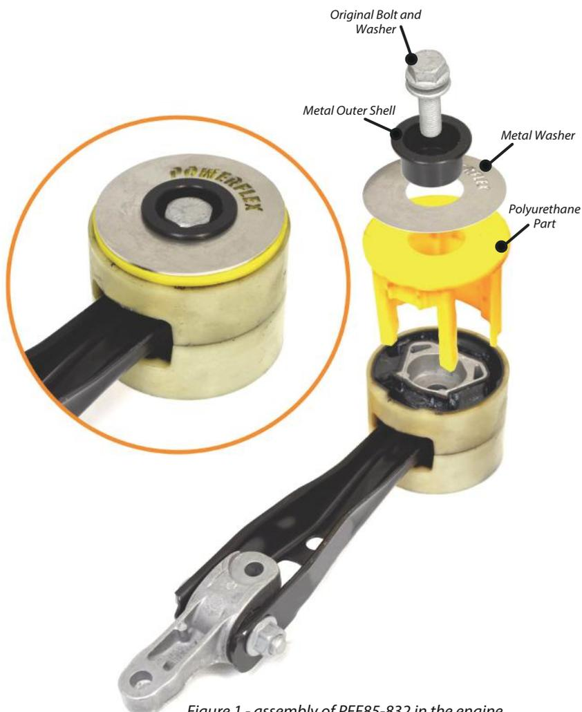
Figure 1 - assembly of PFF85-832 in the engine mount
